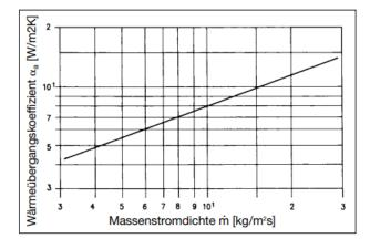
Heat transfer coefficient  $\alpha_{a}^{\phantom{\dagger}}$  for Corrofin
